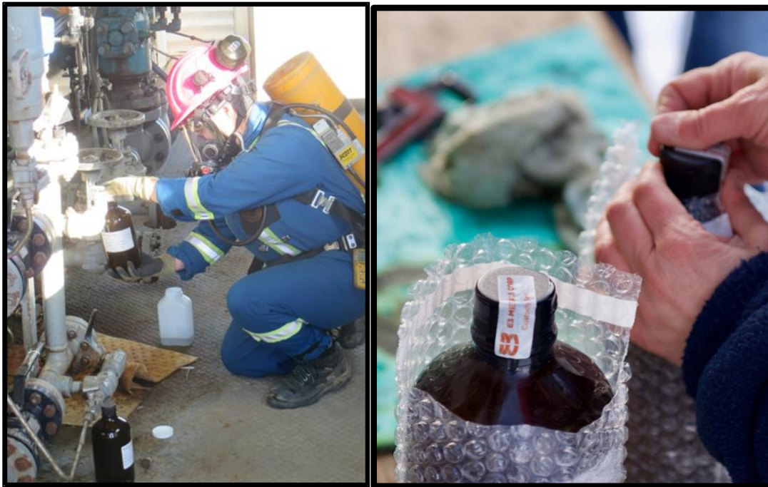
Figure 13. Example of sample collection at a test separator. Left: Maxxam employee collecting sample from test separator access port. Right: Sealed well samples.
