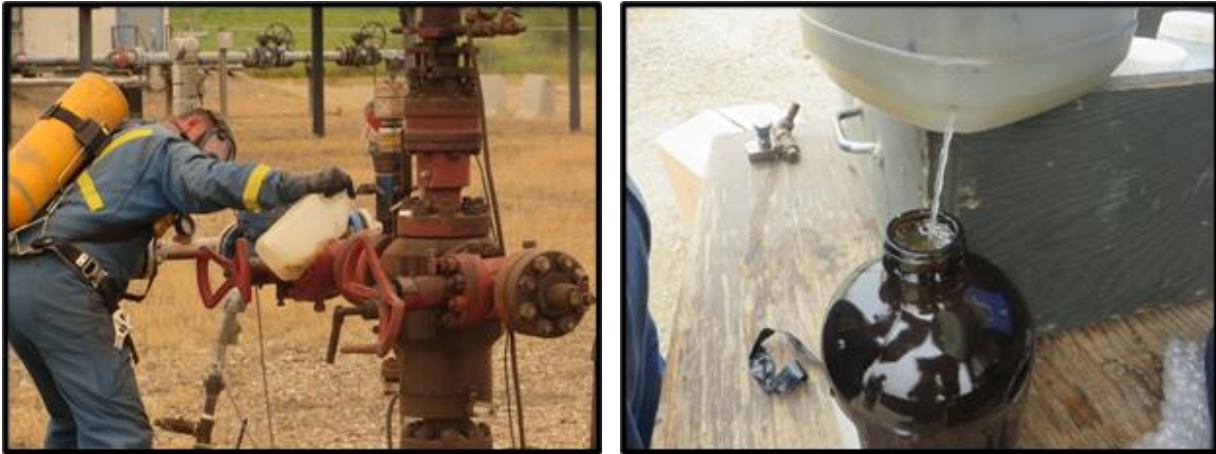
Figure 9-1. Sample collection at wellhead. Left: Maxxam employee sampling from access port into 4 L plastic container. Right: Decanting brine sample from bottom of 4 L container.
